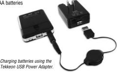
3. Plug the USB plug on the opposite end of the input/output cord into a USB port on a computer or a USB power adapter (such as Tekkeon's myCharger, MP1650). The charging lamp will light as follows to indicate the battery status:
